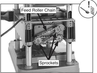
**Figure 25.** Cutterhead elevation leadscrews and feed roller drive chain exposed for lubricating.
